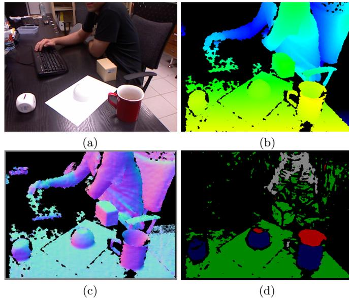
**Fig. 4.** Illustration of the pointcloud segmentation process: (a) example image, (b) the raw depth map, (c) normal vector map, (d) segmented point clouds
