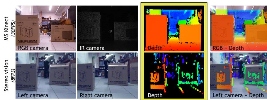
**Fig. 1.** Comparison of depth maps generated from MS Kinect and stereo vision algorithm from OpenCV library
