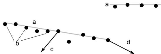
**Fig. 2.** Some caveats of estimating normals from sampled points; a - parts of real surfaces, b - sampled points, c - incorrect normal due to presence of noise, d - incorrect normal on edge of surface
