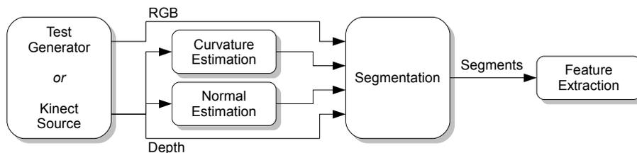
Fig. 3. The proposed segmentation processing pipeline
