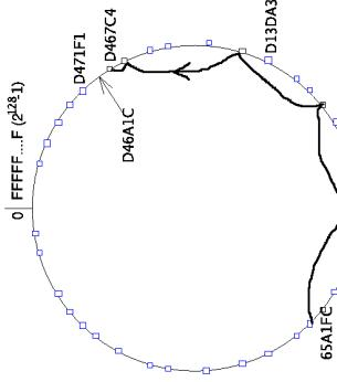
Black color depicts live nodes. The space is considered as circular: node 0 is adjacent to node  $(2^{128} - 1)$ . The diagram illustrates the routing of a message from node 65A1FC to D46A1C using leaf set information alone, assuming leaf sets of size 8 ( $l = 4$ , in Pastry usually 8). This is a degenerate type of routing that would scale very poorly; it is not used in practice.
