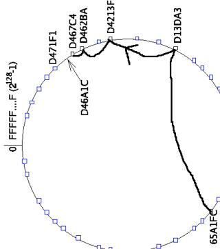
Routing a message from node 65A1FC to D46A1C. With the aid of a well-populated routing table the message can be delivered in  $\log_6(N)$  hops.
