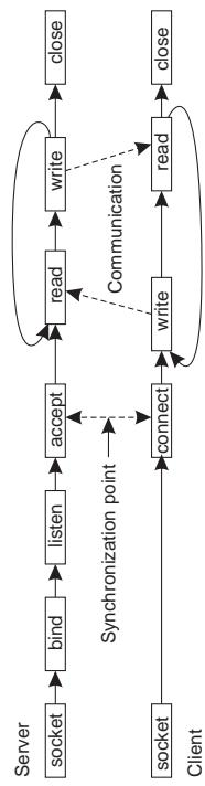
Connection-oriented communication pattern using sockets.
