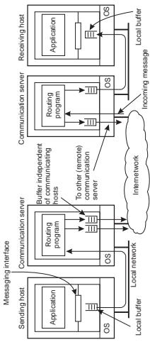
General organization of a communication system in which hosts are connected through a network.
