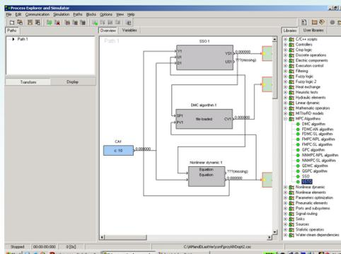
The set-point optimization structures are *computationally efficient* because *linear programming* is used on-line rather than *difficult nonlinear optimization*
