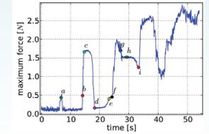
**The plot of total force acting on the tactile sensors**
