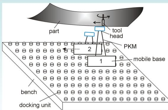
Active mobile fixture system for drilling and milling processes:
