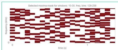
A spectrogram mask for extraction of a single source
