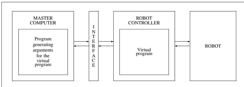
Figure 5.7. The WUT robot system executing TORBOL programs
