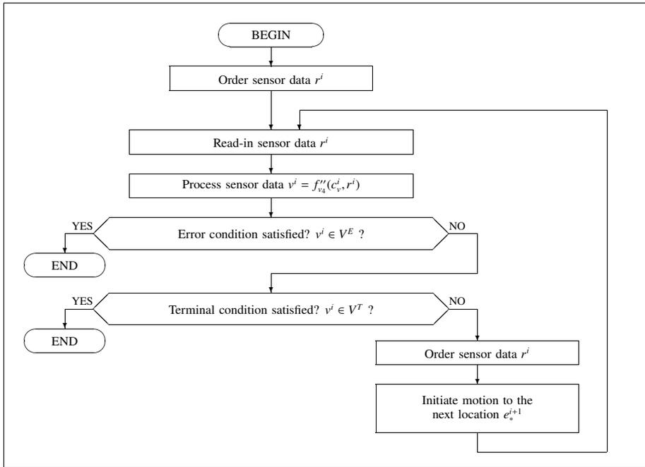
Figure 5.2. Error and terminal condition monitoring
