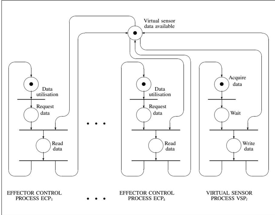
Figure 8.5. Synchronization of several Effector Control Processes with a Virtual Sensor Process (Petri net with initial marking)
