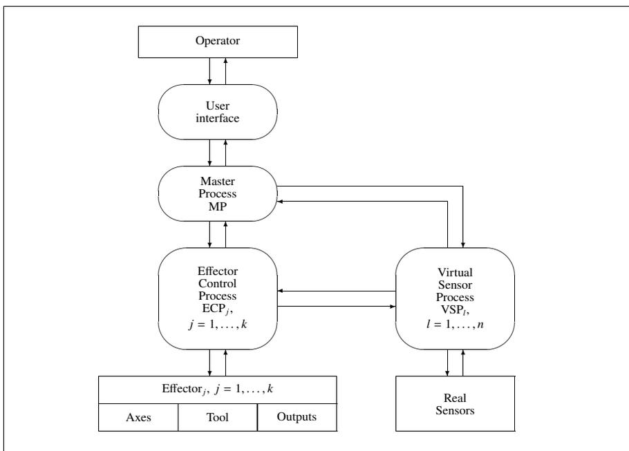
Figure 8.1. Software structure of the system with a Master Process – hierarchical structure
