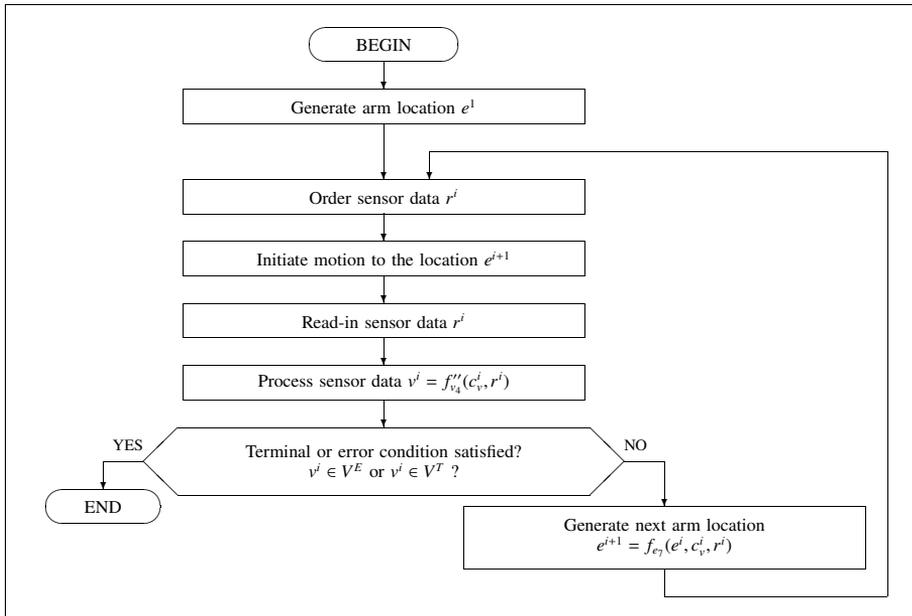
Figure 5.3. The monitoring of current states and control of future states
