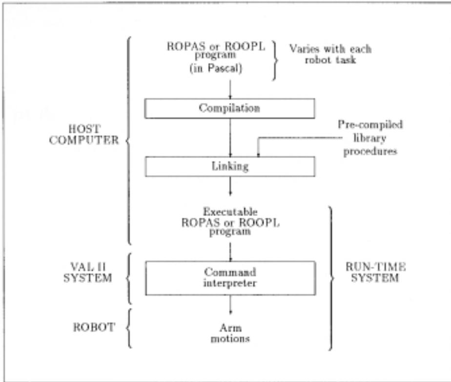
Figure 5.5. Method of processing a ROPAS or ROOPL program
