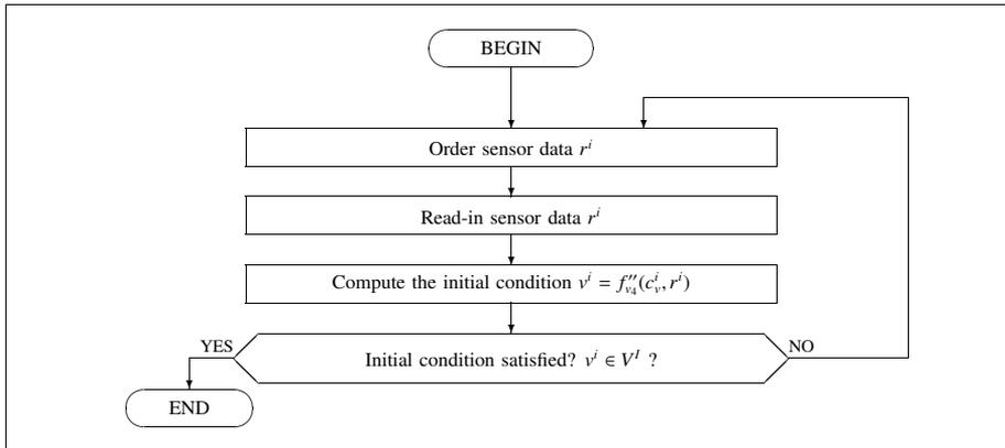
Figure 5.1. Initial condition monitoring
