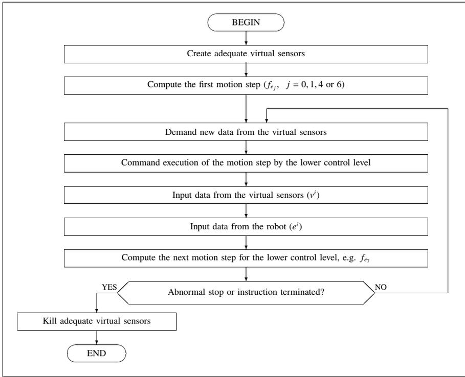
Figure 6.6. Generic structure of the MOVE procedure
