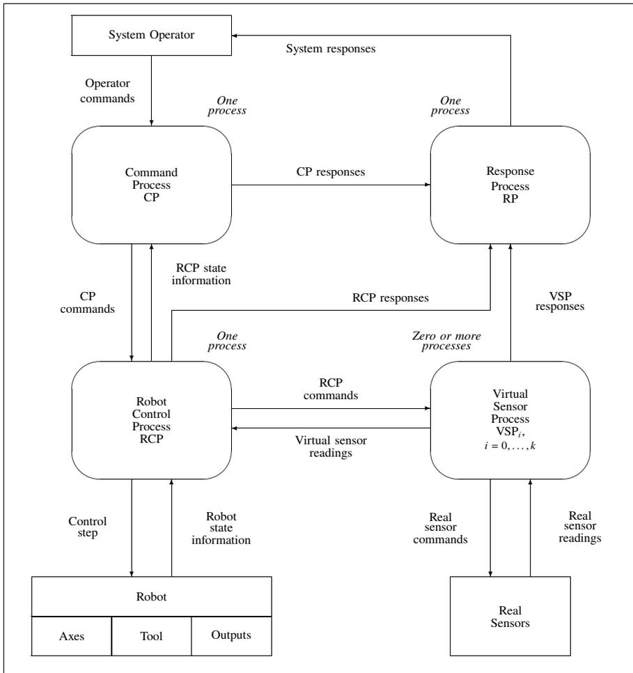
Figure 6.3. Logical structure of the system — process interactions
