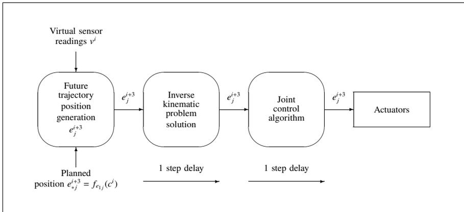
Figure 8.7. Partitioning of an Effector Control Process into a three-stage pipelined structure
