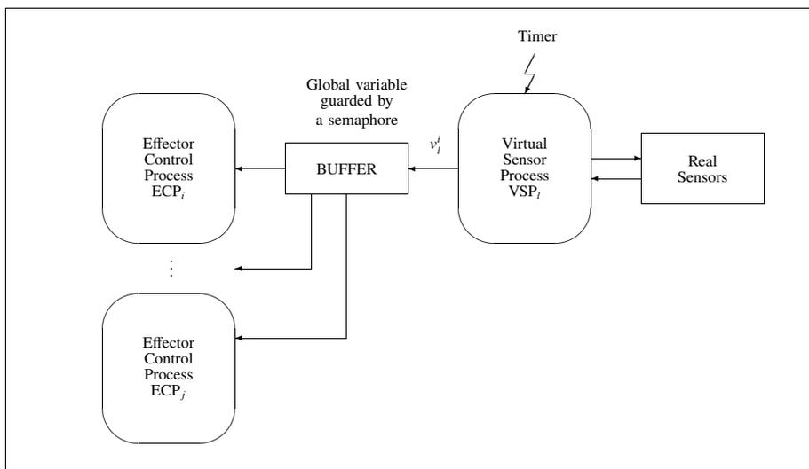
Figure 8.4. Non-interactive method of reading sensor data
