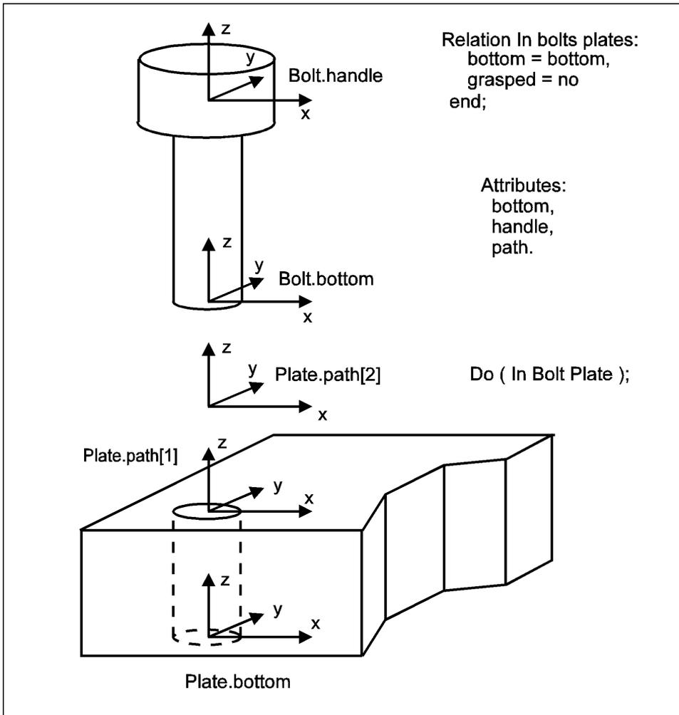
Figure 3.1. Definition of the relation In between a Bolt and a Plate
