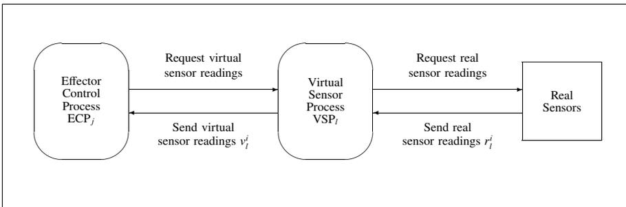
Figure 8.3. Interactive method of reading sensor data through data pipelines
