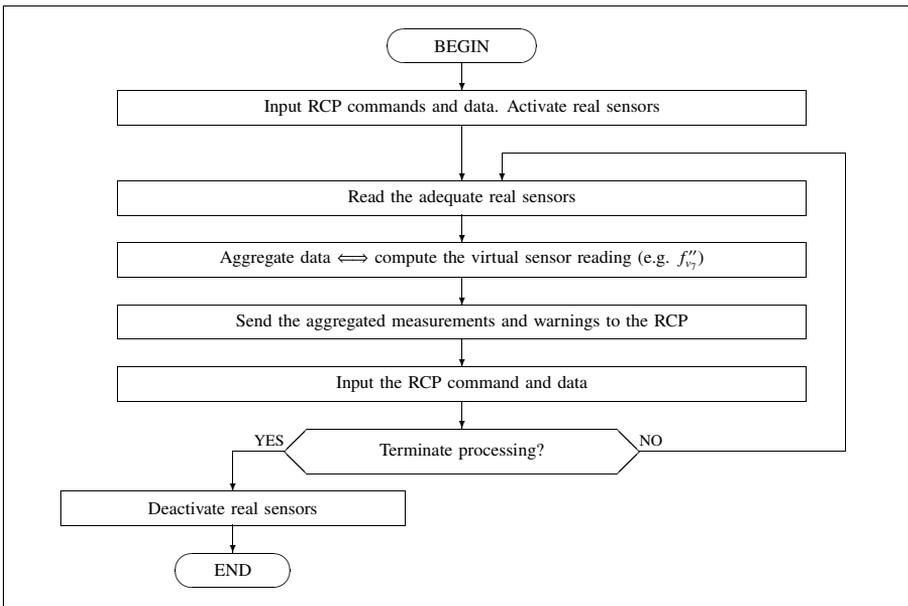
Figure 6.5. Generic structure of the Virtual Sensor Process VSP
