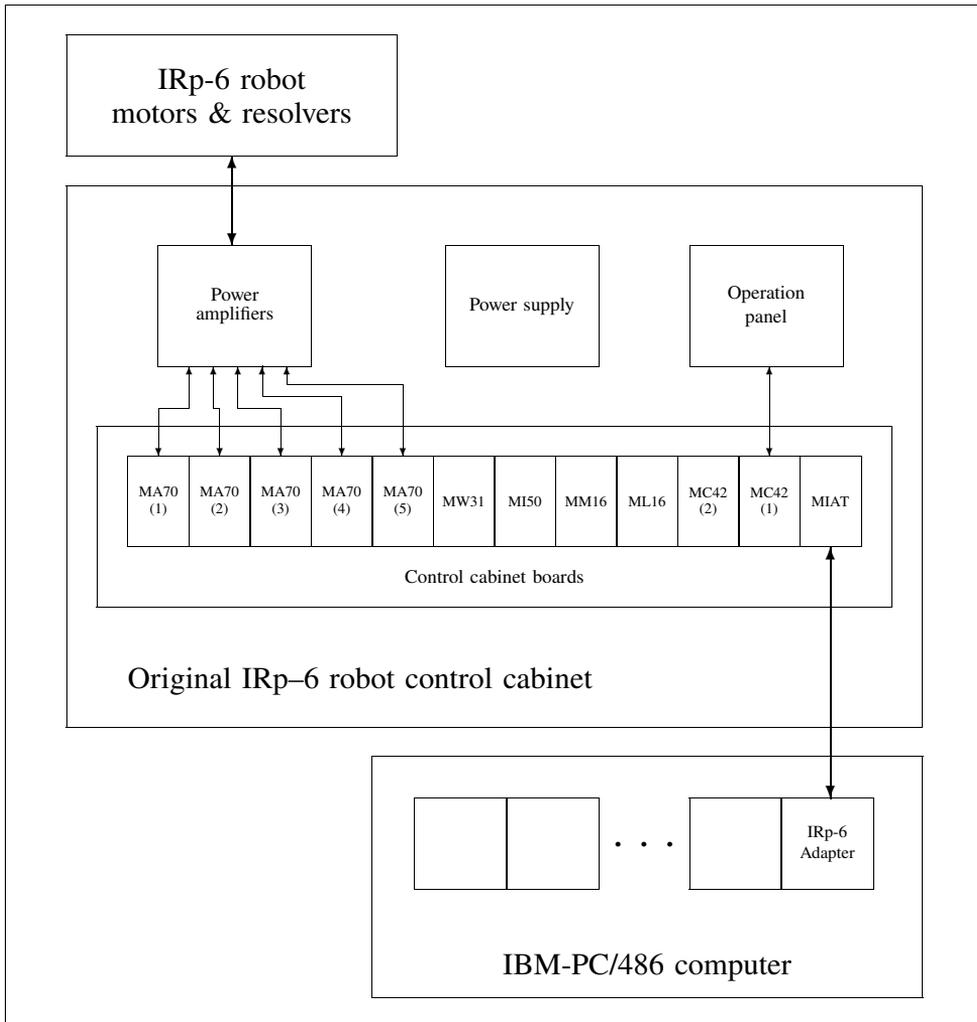
Figure 6.1. Hardware structure of the system
