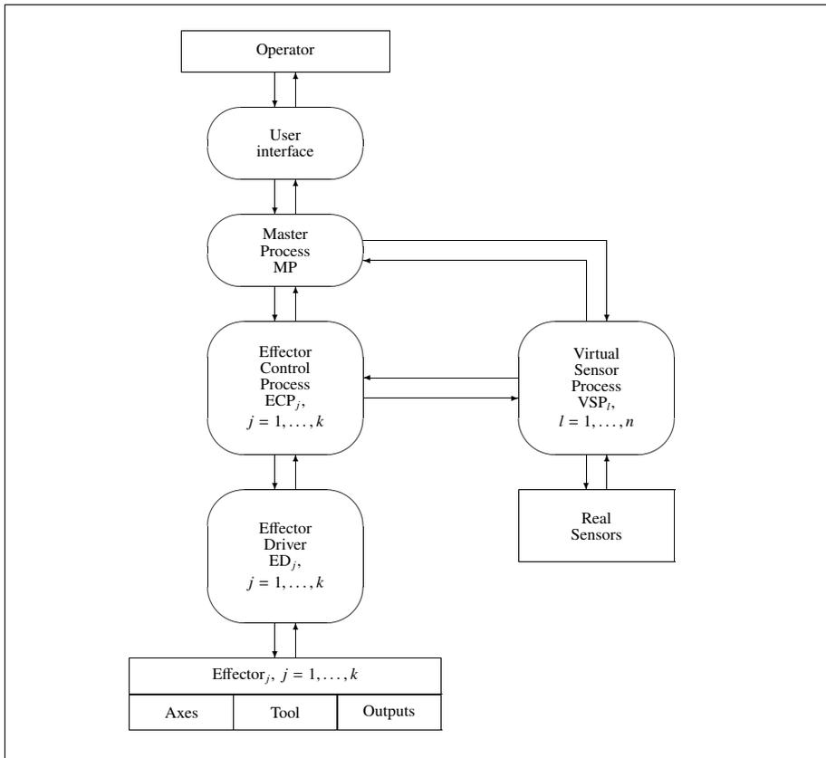
Figure 8.6. Hierarchical structure with an effector driver
