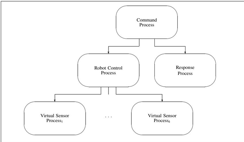
Figure 6.4. Hierarchical dependence of system processes
