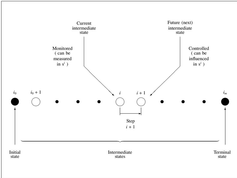
Figure 4.1. Evolution of the system state during execution of a motion instruction
