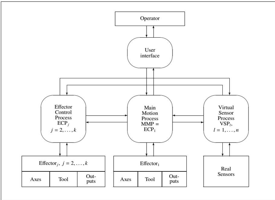
Figure 8.2. Software structure of the system with one of the effector control processes distinguished as a Main Motion Process – flat structure
