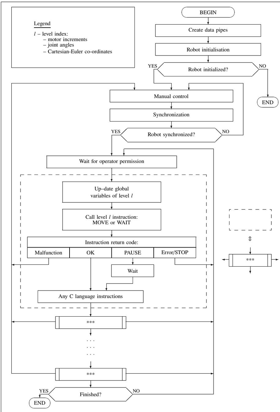
Figure 6.9. Method of creating the Robot Control Process
