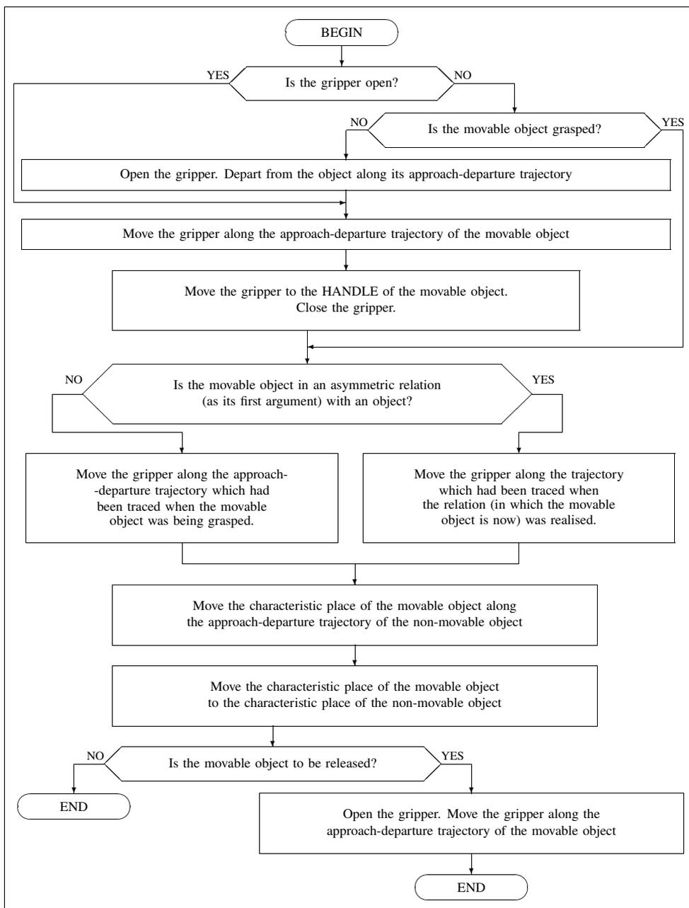
Figure 3.2. Flowchart of the execution of a binary relation
