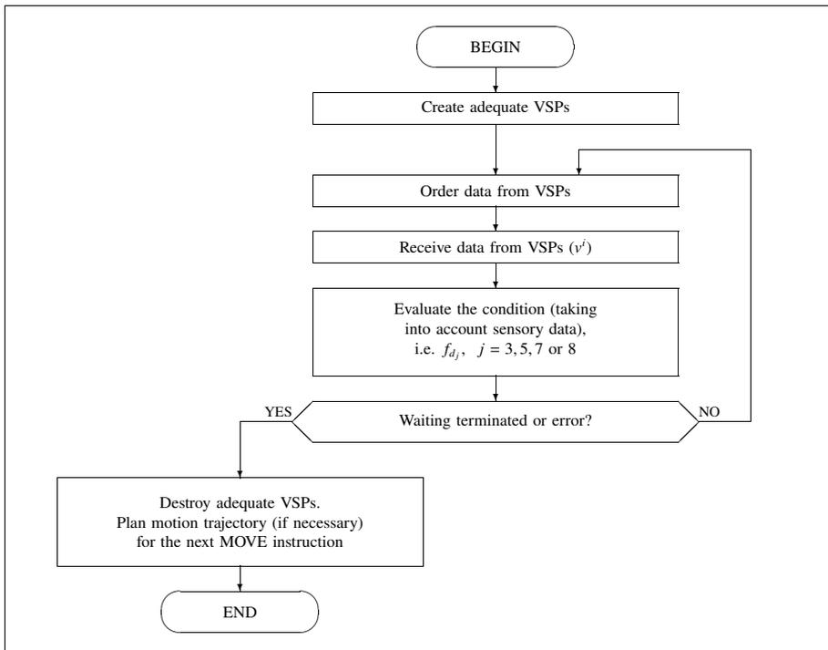
Figure 6.8. Generic structure of the WAIT procedure
