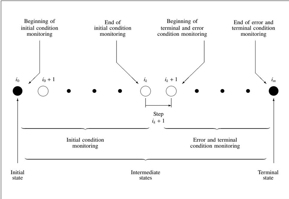
Figure 4.2. Monitoring the execution of a motion instruction
