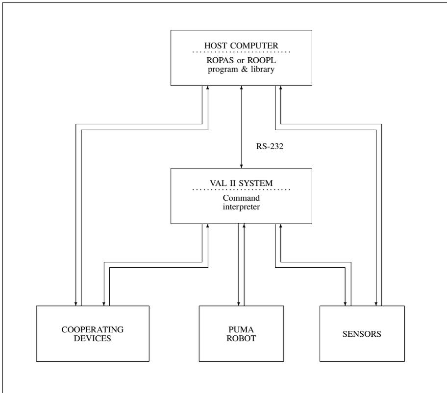
Figure 5.4. Structure of the system executing ROPAS and ROOPL programs
