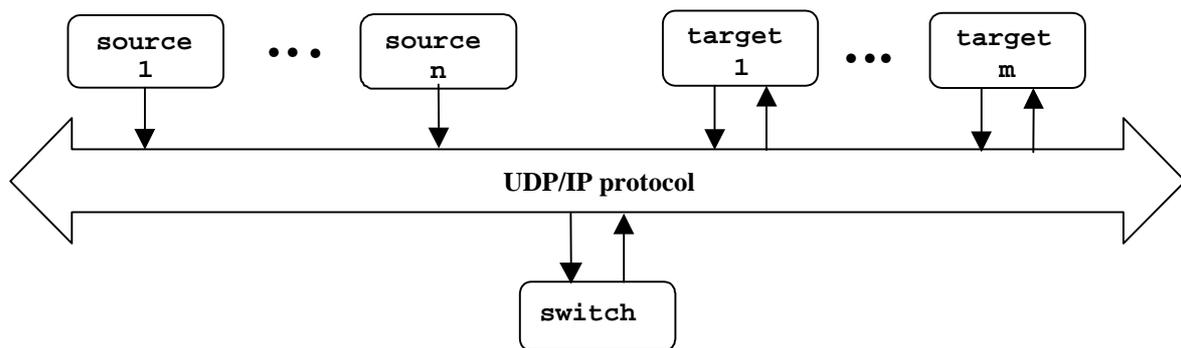
Fig.1 Network Communication of Data Sources And Targets
