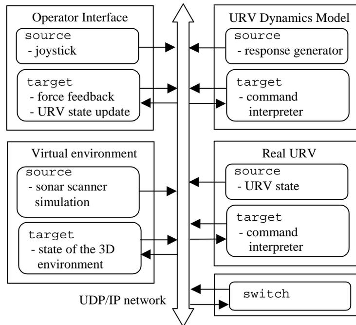
Fig.4. URV control and simulation system structure
