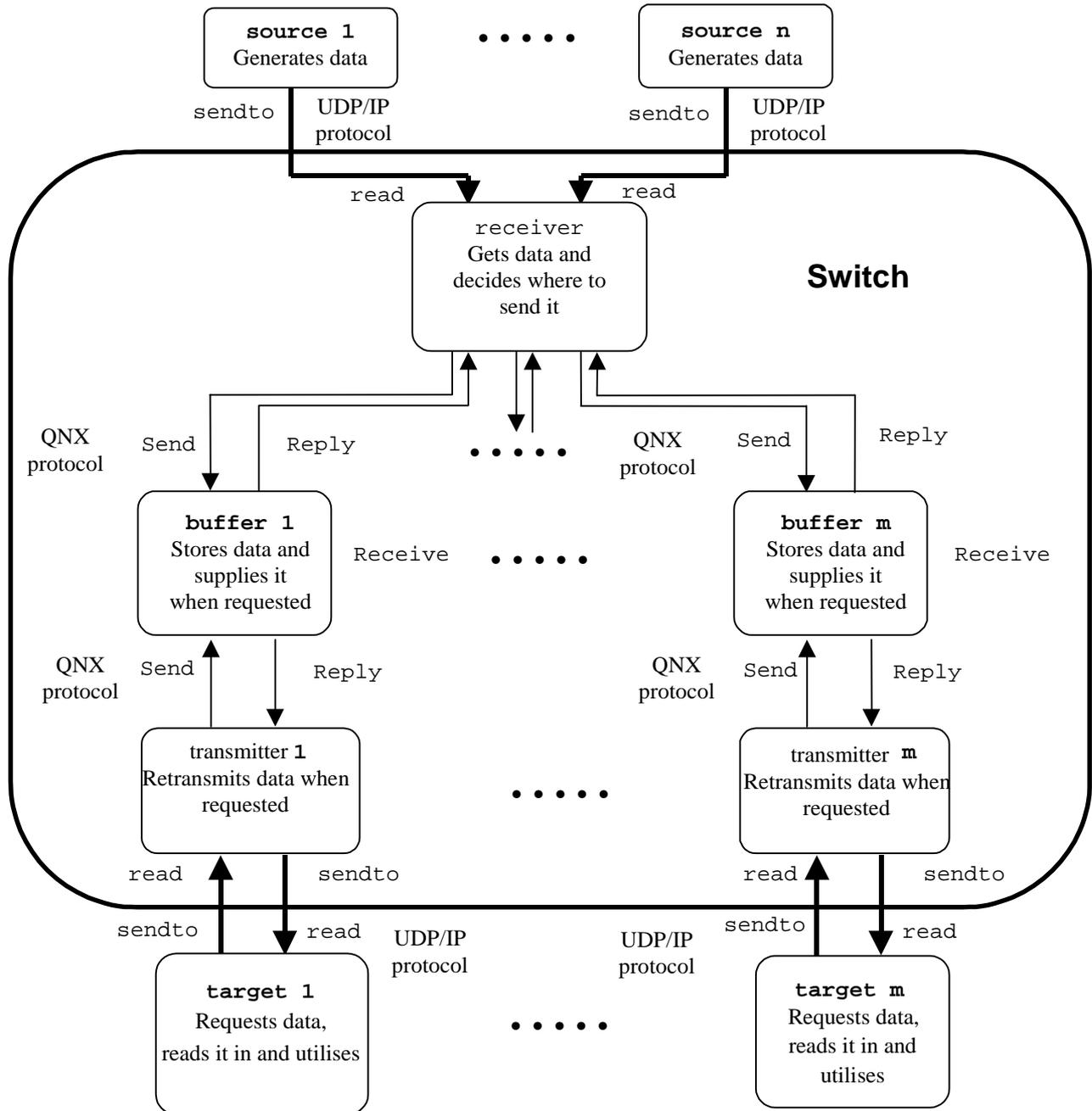
Fig.2 Internal Structure of the Communication Switch
