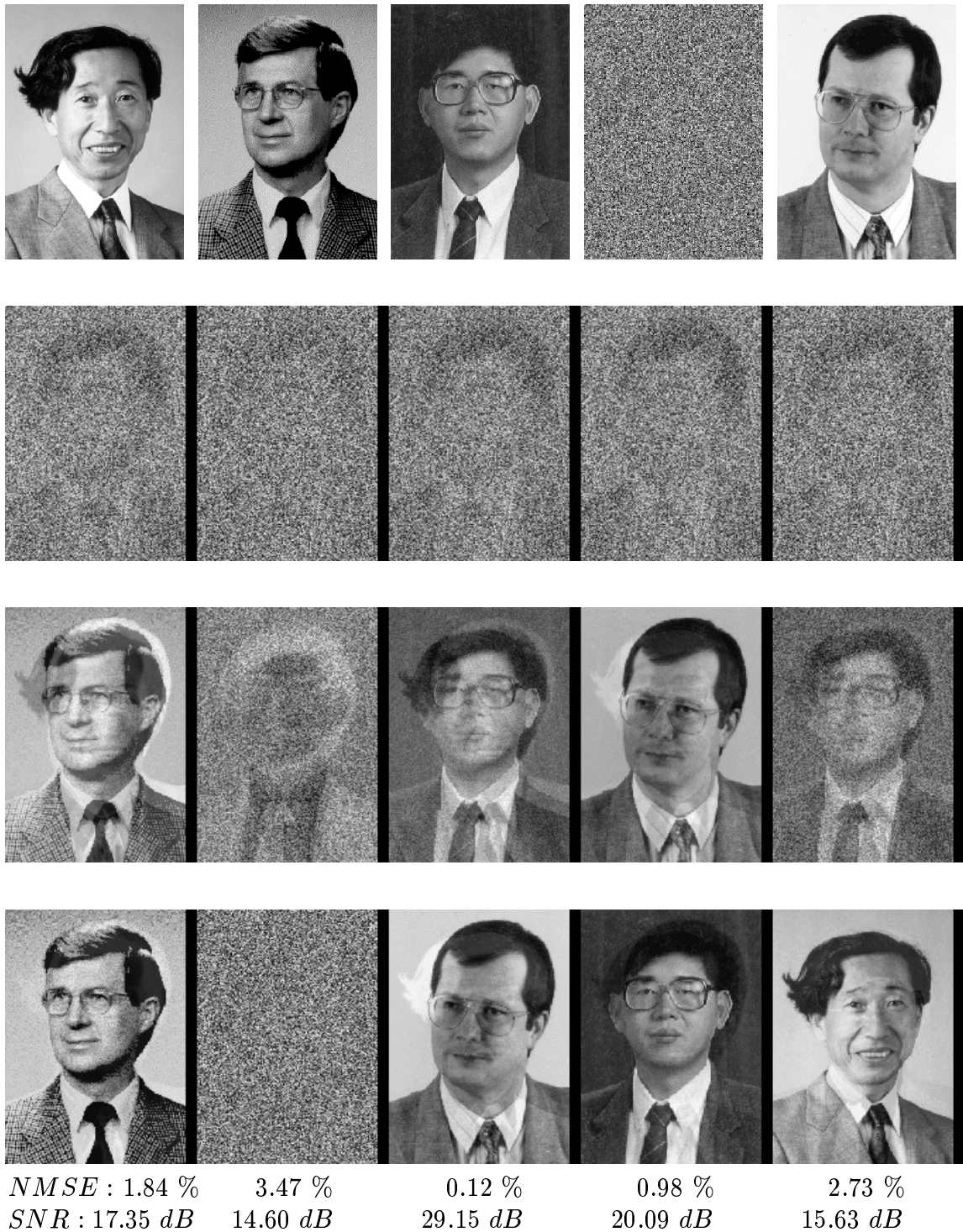
Fig. 2. A mixing and separation of natural face images and Gaussian noise: (top row) five original images (but unknown to the neural net), (second row) five input images for separation, (third row) separation results after three layers, (bottom row) five separated images after five layers ( PI = 0.144 ).
