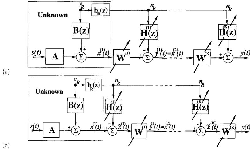
Fig. 5. Alternative improved multi-layer neural network models for blind separation with noise cancellation.
