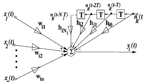
Fig. 3. Simple model of single neuron for simultaneous blind extraction and noise cancellation.
