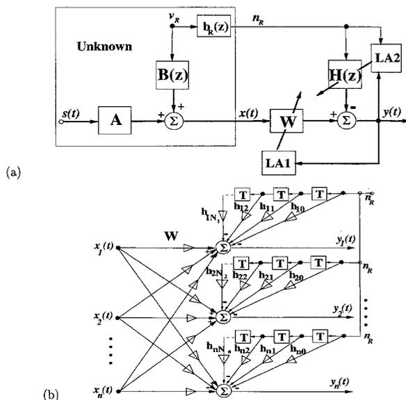
Fig. 2. The basic de-mixing model. (a) Applying two learning algorithms  $LA1$ ,  $LA2$  simultaneously, (b) detailed structure of the de-mixing and de-noising models.
