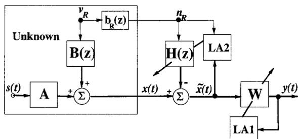
Fig. 4. Alternative (simplified) model for blind separation with noise cancellation as pre-processing.
