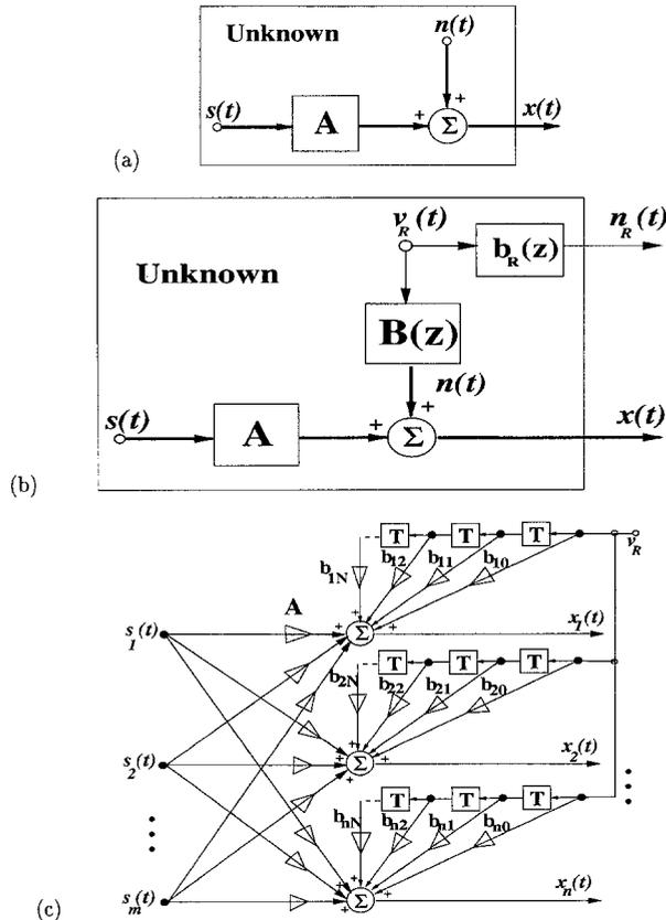
**Fig. 1.** The model of source mixing with additive noise. (a) General model, (b) a mixing model with convolutive noise, (unknown environment noise and its secondary (convolutive) reference noise), (c) more detailed model of the additive convolutive noise.
