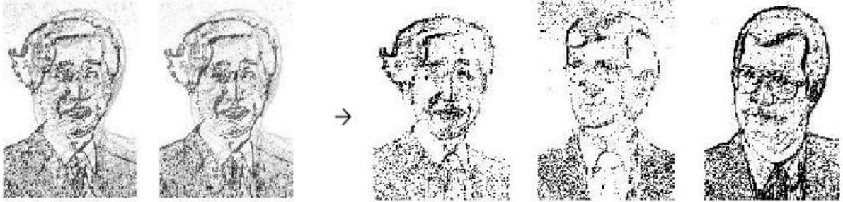
Figure 1: Blind extraction of three sparse sources (binary images) from their two mixtures.
