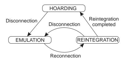
The state-transition diagram of a Coda client with respect to a volume.
