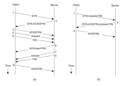
(a) Normal operation of TCP. (b) Transactional TCP.
