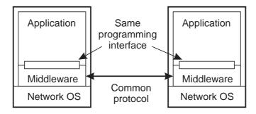
In an open middleware-based distributed system, the protocols used by each middleware layer should be the same, as well as the interfaces they offer to applications.
