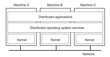
General structure of a multicomputer operating system.
