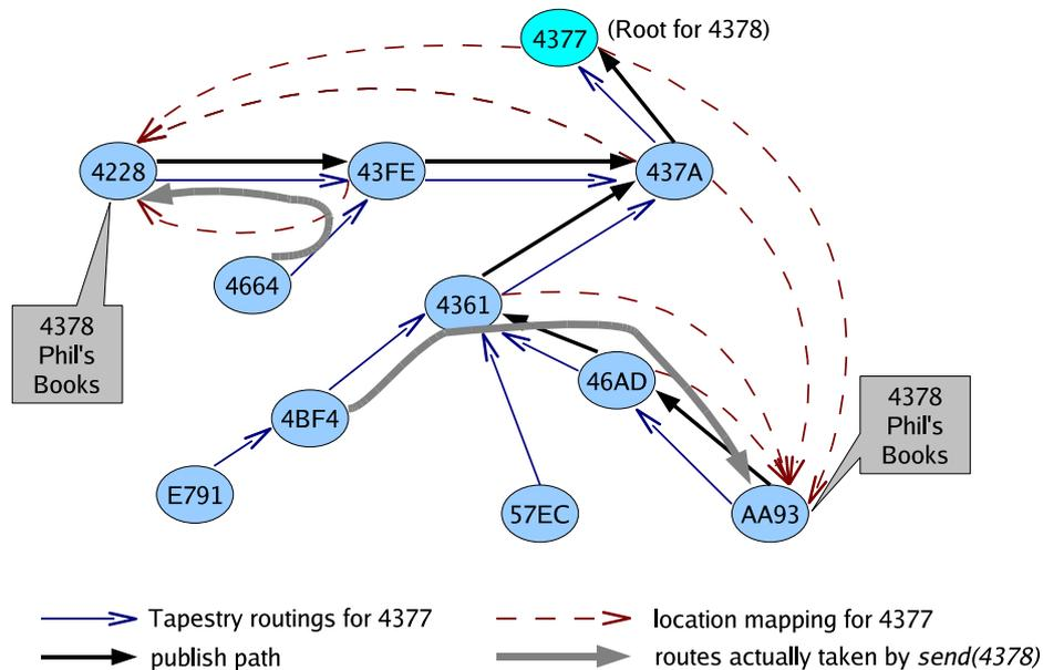
Replicas of the file *Phil's Books* ( $G=4378$ ), hosted at nodes 4228 and AA93. Node 4377 is the root node for object 4378. Shown routings are some of the entries in routing tables. The location mapping (cached while servicing publish messages) are subsequently used to route messages sent to 4378.
