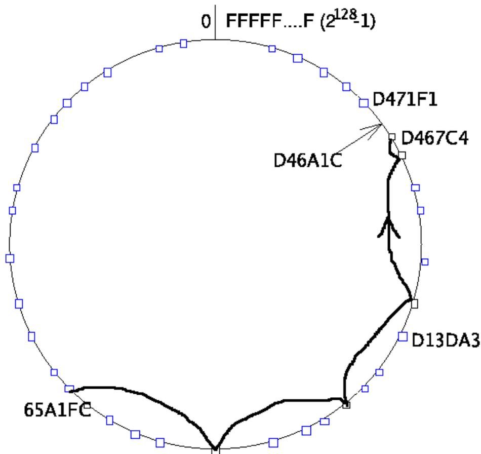
Black color depicts live nodes. The space is considered as circular: node 0 is adjacent to node  $(2^{128} - 1)$ . The diagram illustrates the routing of a message from node 65A1FC to D46A1C using leaf set information alone, assuming leaf sets of size 8 ( $l = 4$ , in Pastry usually 8). This is a degenerate type of routing that would scale very poorly; it is not used in practice.
