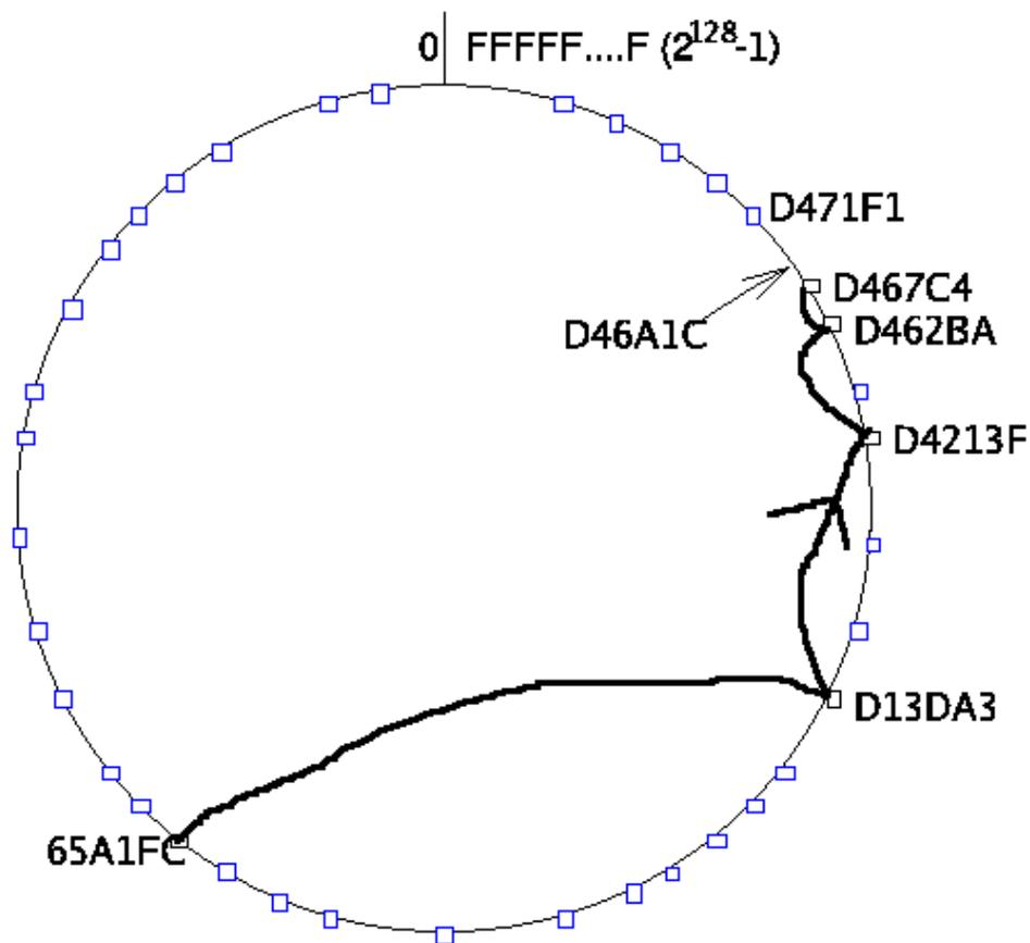
Routing a message from node 65A1FC to D46A1C. With the aid of a well-populated routing table the message can be delivered in  $\log_{16}(N)$  hops.
