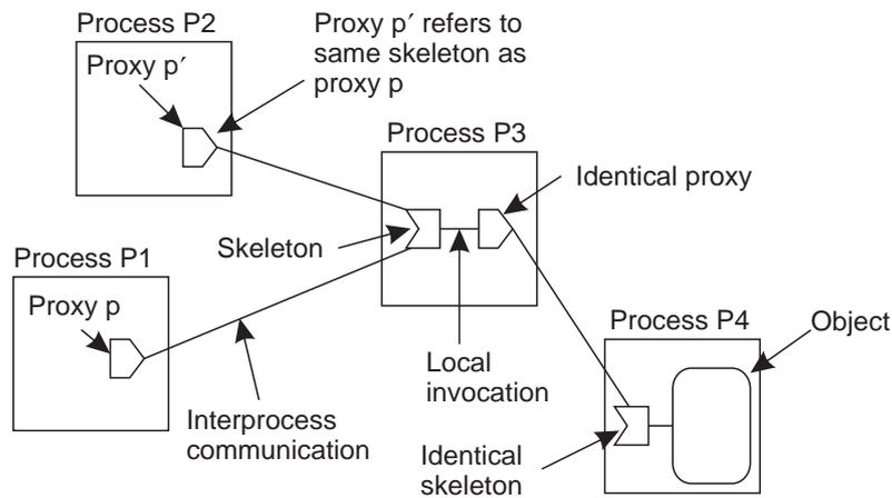
The principle of forwarding pointers using (proxy, skeleton) pairs.
