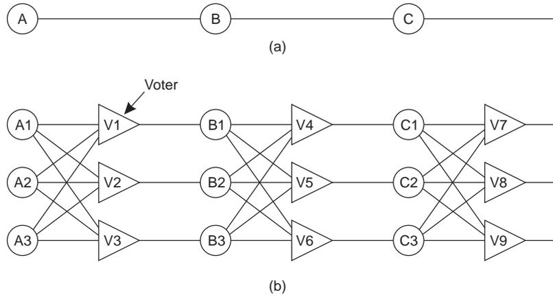
Triple modular redundancy (TMR).
