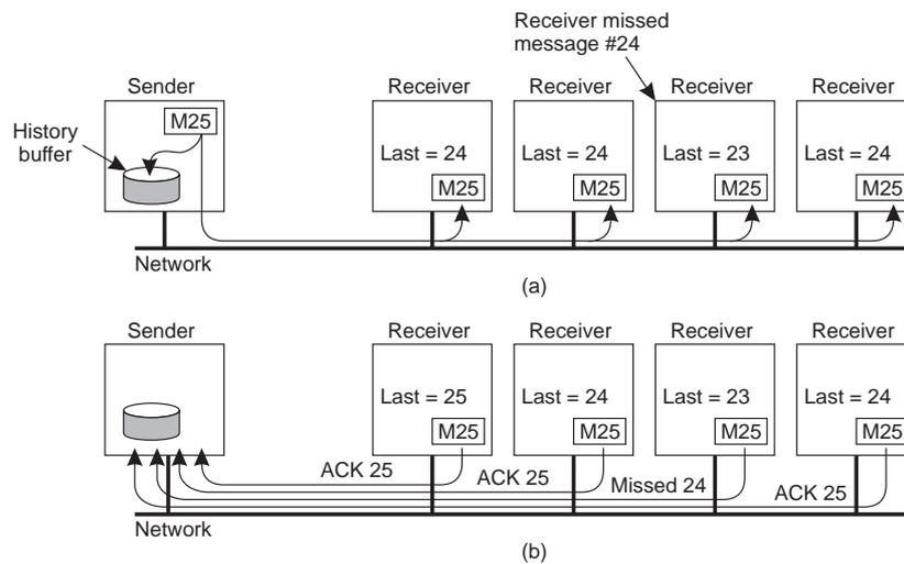
A simple solution to reliable multicasting when all receivers are known and are assumed not to fail: (a) message transmission and (b) reporting feedback.
