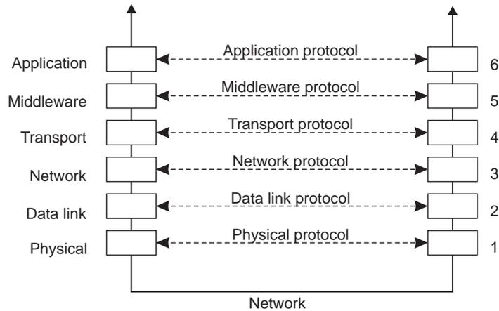
An adapted ISO OSI reference model for networked communication.
