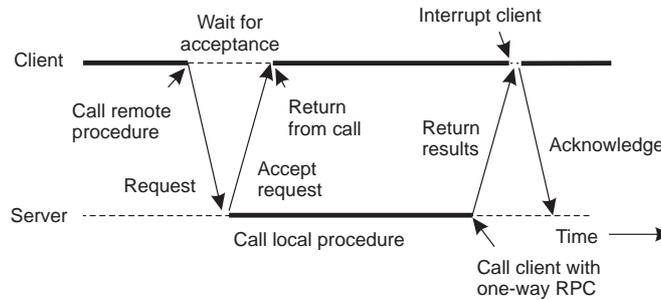
**deferred synchronous RPC** – asynchronous RPC with second call done by the server,
