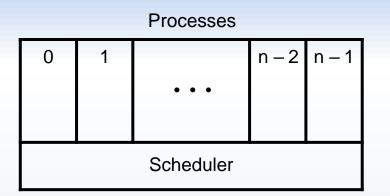
The lowest layer of a process-structured operating system handles interrupts and scheduling. Above that layer there are sequential processes. For processor allocation for particular processes a piece of an OS kernel called **scheduler** is responsible.
