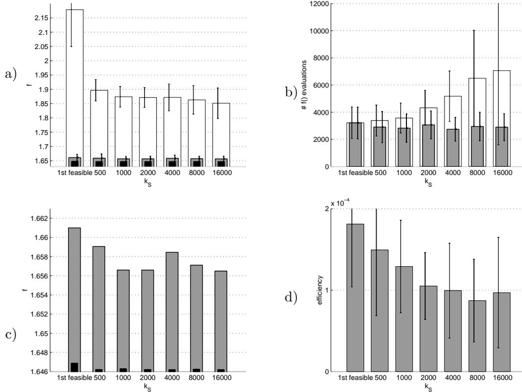
**Figure 8:** Selected statistics for operation of CRS2/COMPLEX hybrid optimisation algorithm. Bars indicate average values; lines attached to bars indicate standard deviations from the average values. Results are drawn for varying switching criterion  $k_S$  — the number of  $f(\cdot)$  evaluations after which a switchover from CRS2 to COMPLEX is performed.
