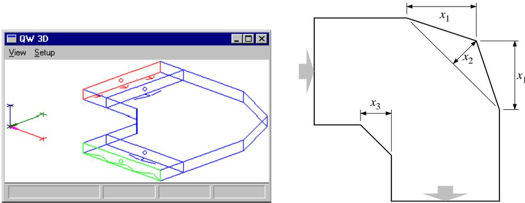
**Figure 5:** Three-dimensional (left) and top (right) view of the waveguide bend subject to design optimisation.
