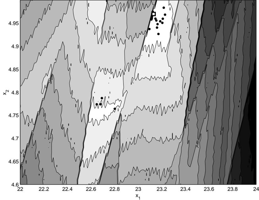
**Figure 9:** Location of CRS2 (black dots) and Powell (white square) solutions for the simplified waveguide design problem on the contour plot of performance index. White areas denote regions of good performance (low value of the performance index).
