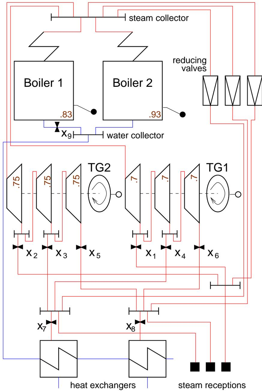
**Figure 11:** The diagram of test power system that is a simplified version of the plant model.
