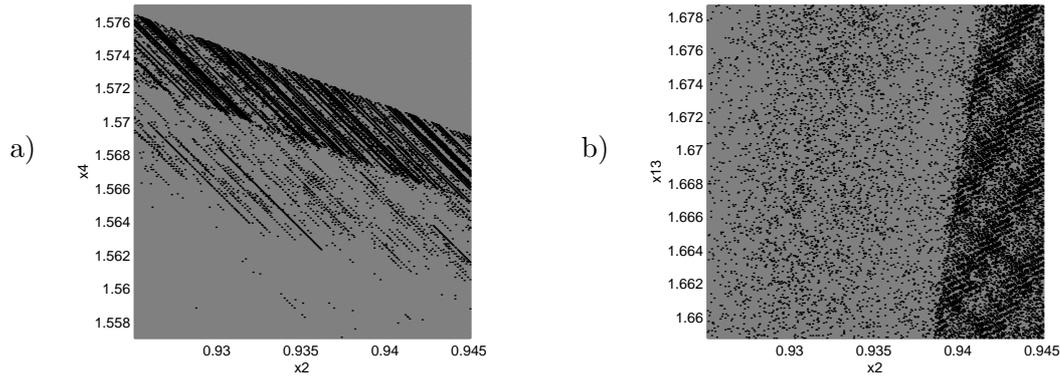
**Figure 1:** Two-dimensional exemplary cuts through  $D_{\mathbf{x}}$  with sets of decision variables values for which the modelling (i.e. computing of  $\mathbf{y}$  by simulation) fails marked with black colour.
