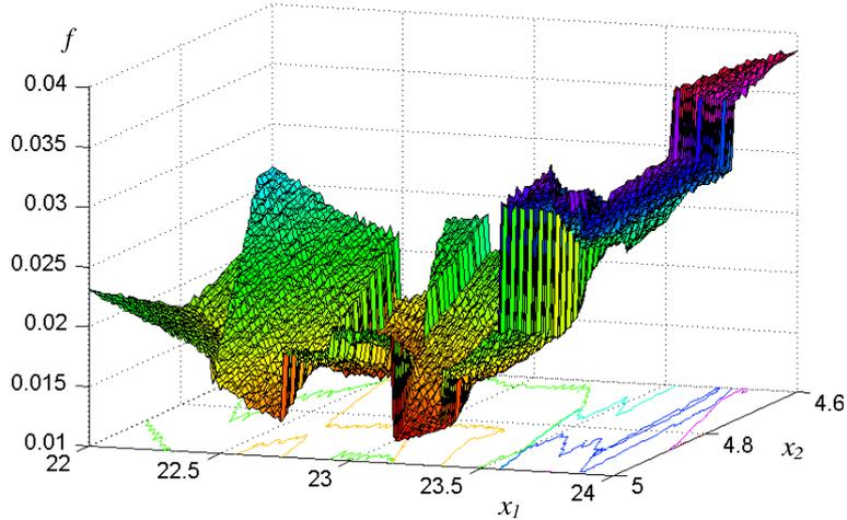
**Figure 6:** Fragment of performance function surface for waveguide bend design optimisation problem.
