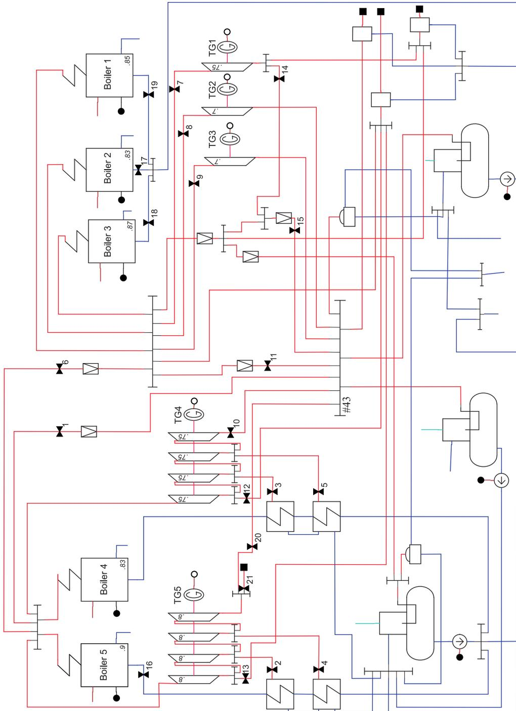
**Figure 10:** The diagram of industrial power plant at 'Janikosoda' chemical works in Janikowo.
