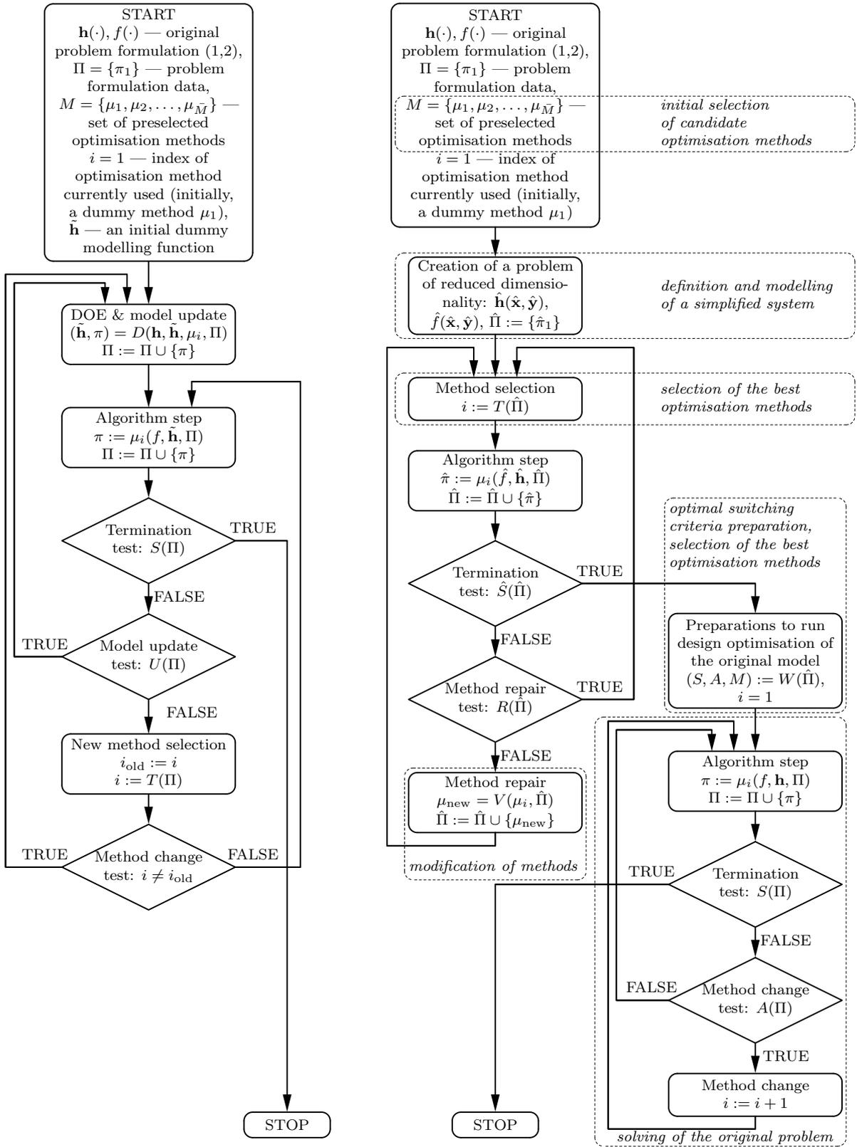
**Figure 12:** Flowcharts for the operation of the standard (left) and the proposed (right) approaches to design optimisation.
