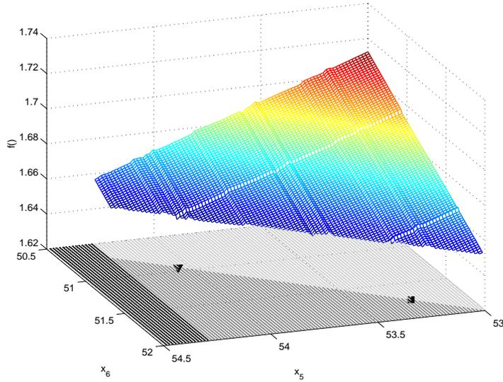
**Figure 7:** Reference locations of the simplified problem solutions in the search subspace of  $x_5$  and  $x_6$  and the performance index surface. (CRS2 solution location is marked with a triangle; Epogy solution is marked with a square.)
