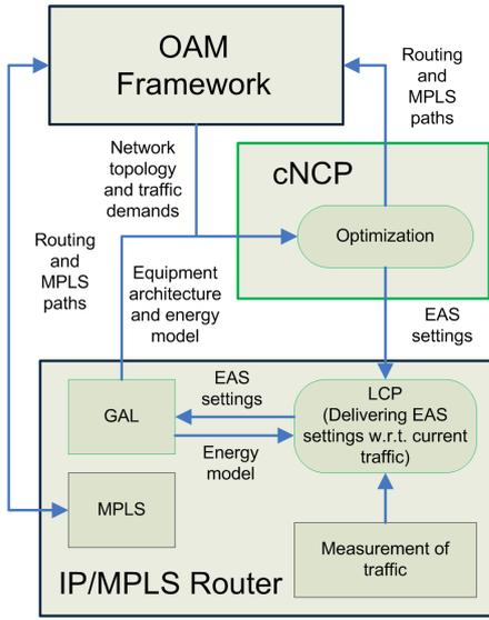
Fig. 1. The architecture of the control framework (centralized control).
