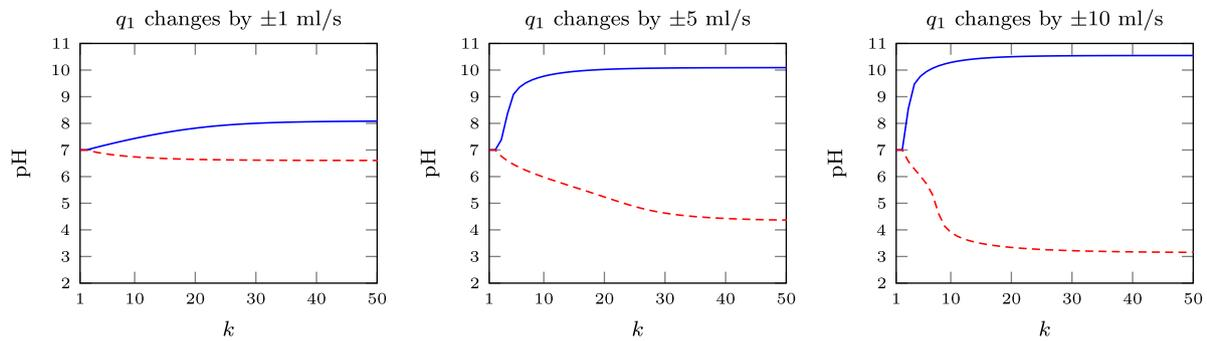
**Fig. 4.** Step-responses of the reactor (the value of pH caused by increasing (solid line) and decreasing (dashed line) the base flow rate  $q_1$  by 1 ml/s (left panel), 5 ml/s (middle panel) and 10 ml/s (right panel) at  $k=1$ ).
