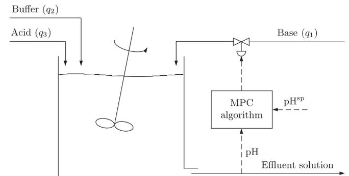
Fig. 2. The structure of the control system of the neutralisation reactor.
