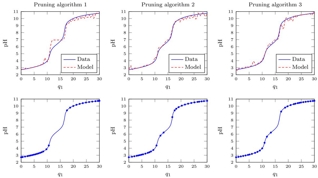
**Fig. 9.** The steady-state validation data set vs. the output of the pruned LS-SVM approximators (top panels) and location of support vectors (bottom panels) obtained by three pruning algorithms;  $\sigma = 0.5$ ,  $n_{sv} = 30$ .
