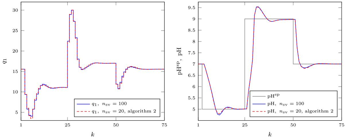
**Fig. 18.** Simulation results of the MPC-NO algorithm based on: the full LS-SVM Wiener model with  $n_{sv} = 100$  support vectors (solid line) and the model with  $n_{sv} = 20$  vectors pruned by the algorithm 2 (dashed line);  $\sigma = 5$ .
