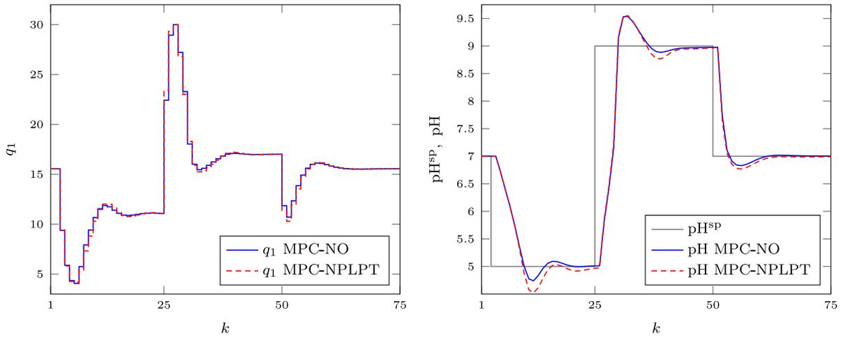
**Fig. 20.** Simulation results: the MPC-NO algorithm (solid line) vs. the MPC-NPLPT algorithm with  $\delta_u = \delta_y = 10$  (dashed line); both algorithms use the same LS-SVM Wiener model with  $\sigma = 5$ ,  $n_{\text{sv}} = 30$ , pruned by the algorithm 2.
