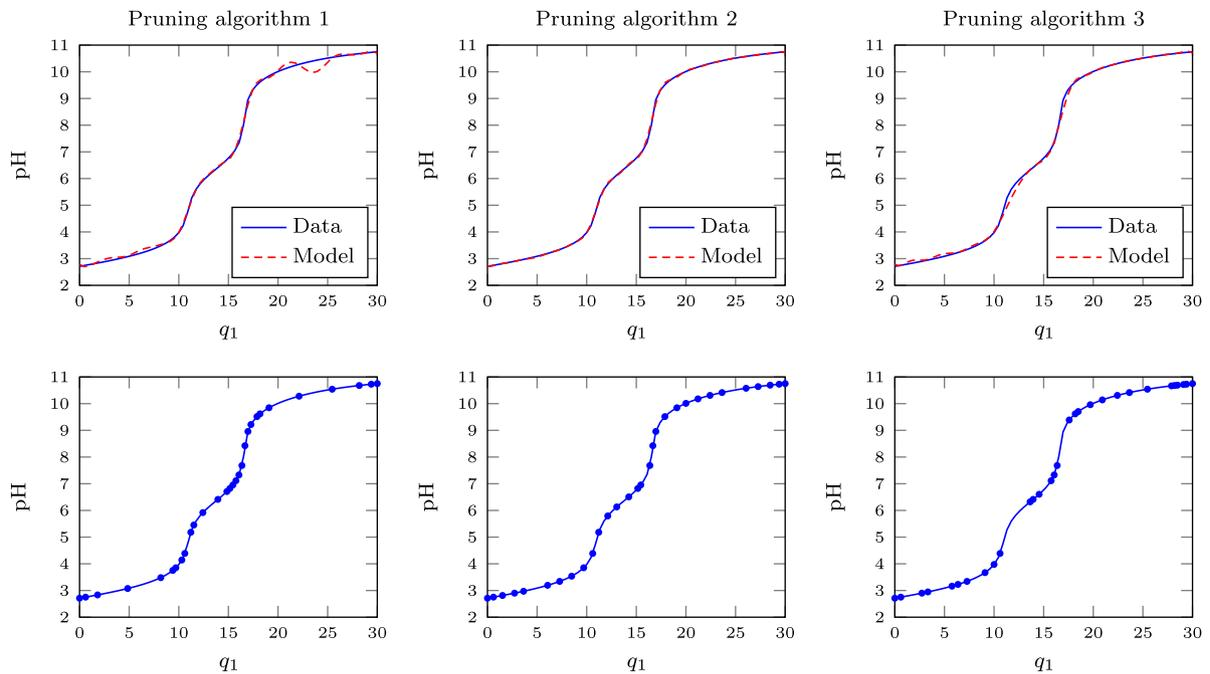
**Fig. 12.** The steady-state validation data set vs. the output of the pruned LS-SVM approximators (*top panels*) and location of support vectors (*bottom panels*) obtained by three pruning algorithms;  $\sigma = 5$ ,  $n_{sv} = 30$ .
