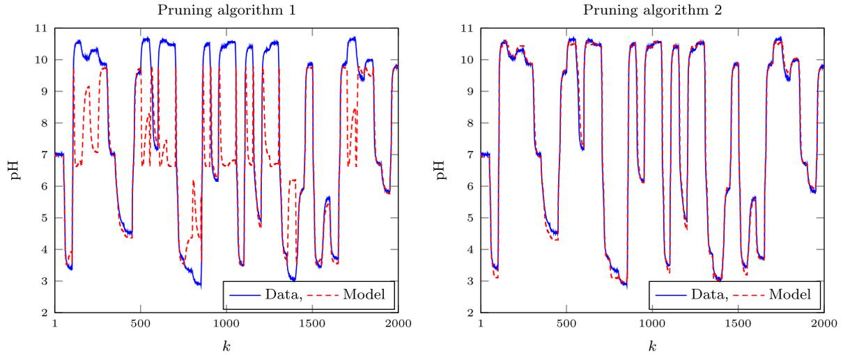
Fig. 15. The dynamic validation data set (solid line) vs. the output of the pruned models obtained by pruning algorithms 1 and 2 (dashed line);  $\sigma = 5$ ,  $n_{sv} = 20$ .
