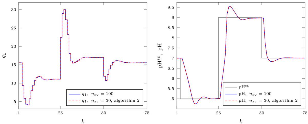
**Fig. 19.** Simulation results of the MPC-NO algorithm based on: the full LS-SVM Wiener model with  $n_{sv} = 100$  support vectors (solid line) and the model with  $n_{sv} = 30$  vectors pruned by the algorithm 2 (dashed line);  $\sigma = 5$ .
