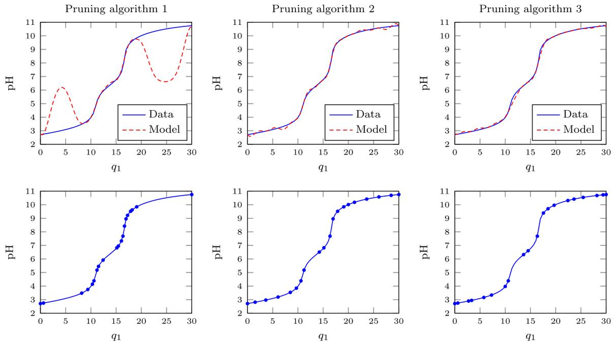
**Fig. 11.** The steady-state validation data set vs. the output of the pruned LS-SVM approximators (*top panels*) and location of support vectors (*bottom panels*) obtained by three pruning algorithms;  $\sigma = 5$ ,  $n_{sv} = 20$ .
