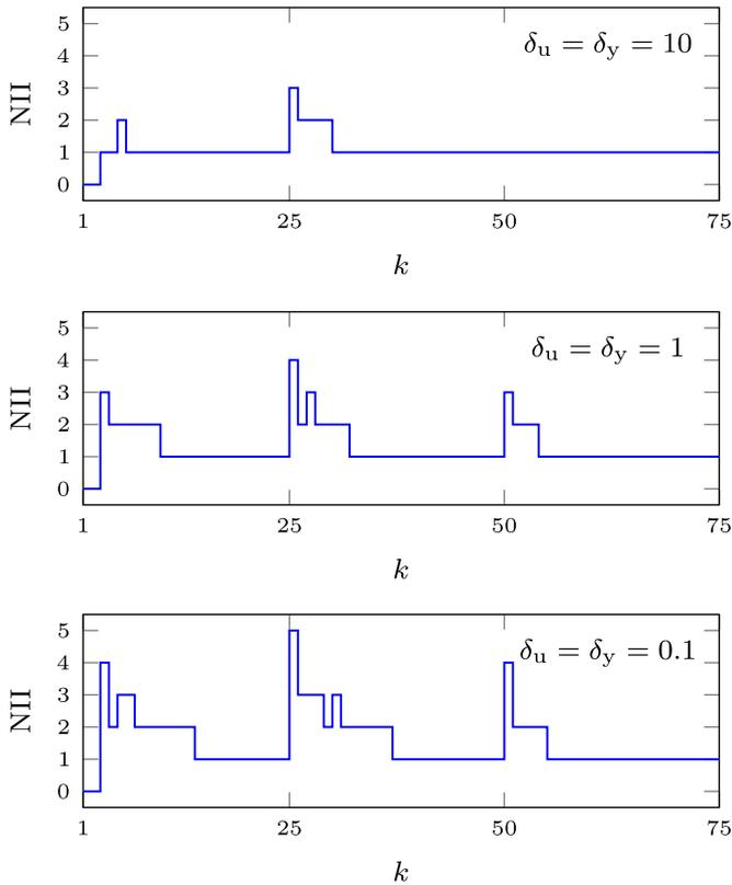
**Fig. 23.** The number of internal iterations NII in the consecutive sampling instants of the MPC-NPLPT algorithm for different values of  $\delta_u = \delta_y$ ; all algorithms use the same LS-SVM Wiener model with  $\sigma = 5$ ,  $n_{sv} = 30$ , pruned by the algorithm 2.
