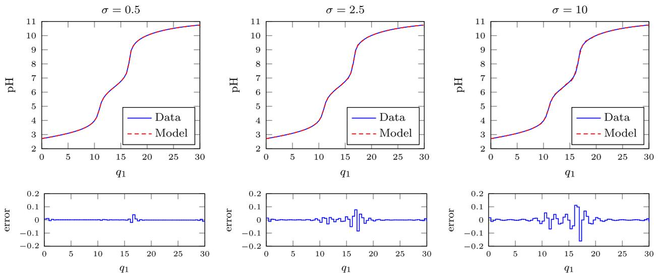
**Fig. 6.** The steady-state validation data set vs. the output of the LS-SVM approximator and model errors for  $\sigma = 0.5$  (left panels),  $\sigma = 2.5$  (middle panels),  $\sigma = 10$  (right panels);  $n_{sv} = 100$ .
