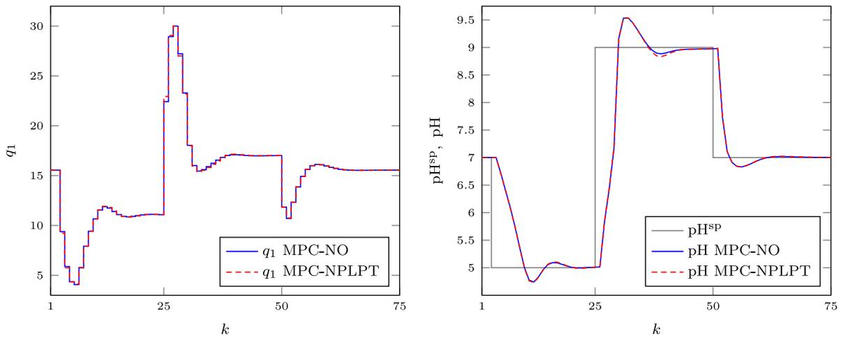
**Fig. 21.** Simulation results: the MPC-NO algorithm (solid line) vs. the MPC-NPLPT algorithm with  $\delta_u = \delta_y = 1$  (dashed line); both algorithms use the same LS-SVM Wiener model with  $\sigma = 5$ ,  $n_{\text{sv}} = 30$ , pruned by the algorithm 2.
