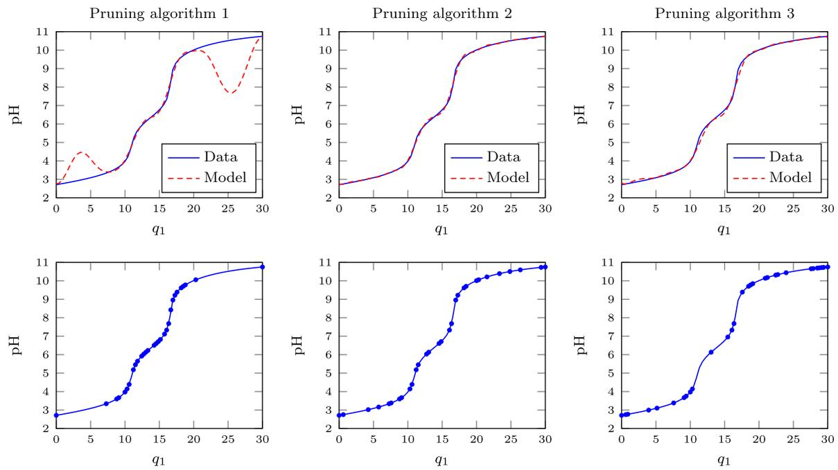
**Fig. 13.** The steady-state validation data set vs. the output of the pruned LS-SVM approximators (top panels) and location of support vectors (bottom panels) obtained by three pruning algorithms;  $\sigma = 10$ ,  $n_{sv} = 30$ .
