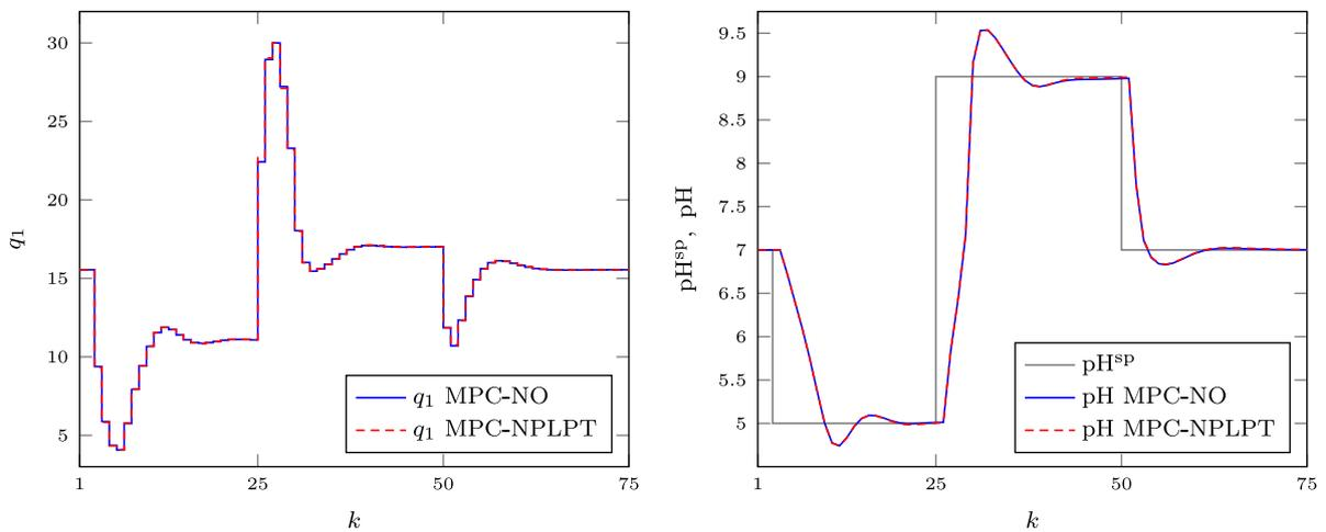
**Fig. 22.** Simulation results: the MPC-NO algorithm (solid line) vs. the MPC-NPLPT algorithm with  $\delta_u = \delta_y = 0.1$  (dashed line); both algorithms use the same LS-SVM Wiener model with  $\sigma = 5$ ,  $n_{\text{sv}} = 30$ , pruned by the algorithm 2.
