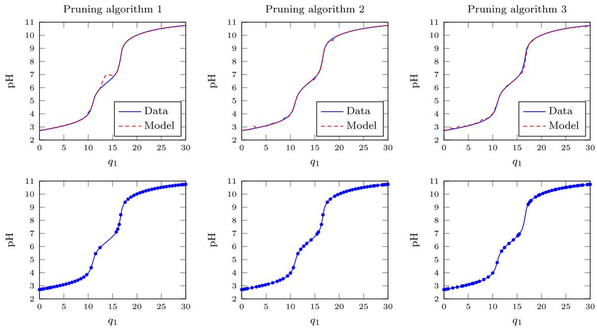
**Fig. 10.** The steady-state validation data set vs. the output of the pruned LS-SVM approximators (top panels) and location of support vectors (bottom panels) obtained by three pruning algorithms;  $\sigma = 0.5$ ,  $n_{sv} = 50$ .
