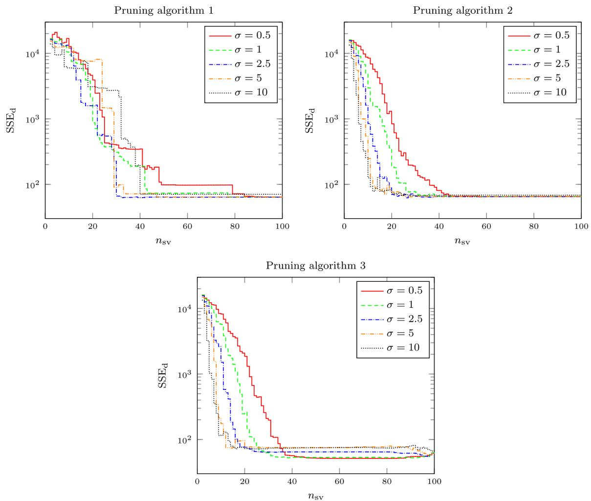
**Fig. 14.** The influence of the number of support vectors  $n_{sv}$  on the error  $SSE_d$  of the LS-SVM Wiener model for the validation data set in three compared pruning algorithms.
