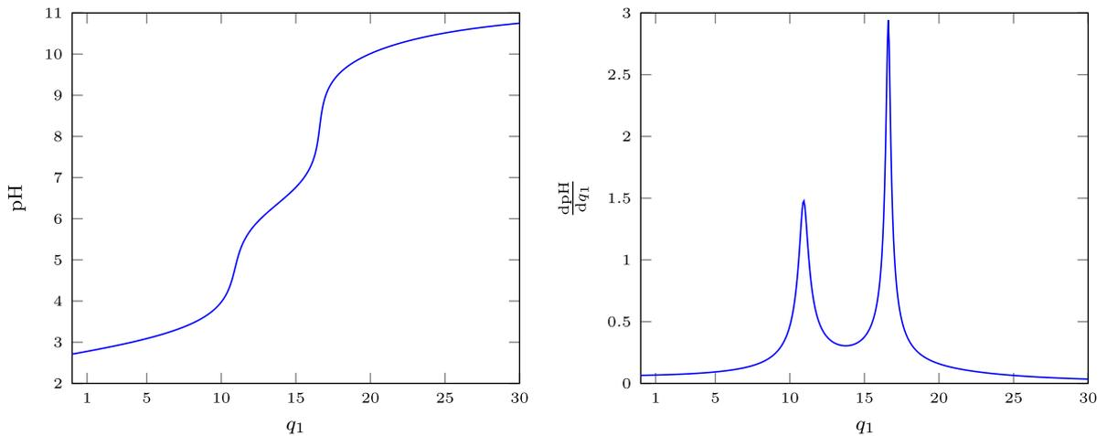
Fig. 3. The steady-state characteristics of the neutralisation reactor (left panel) and its steady-state gain (right panel).
