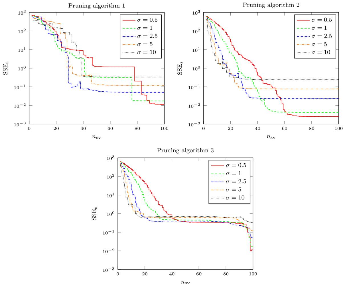
Fig. 8. The influence of the number of support vectors  $n_{sv}$  on the error  $SSE_s$  of the steady-state part of the LS-SVM Wiener model for the validation data set in three compared pruning algorithms.
