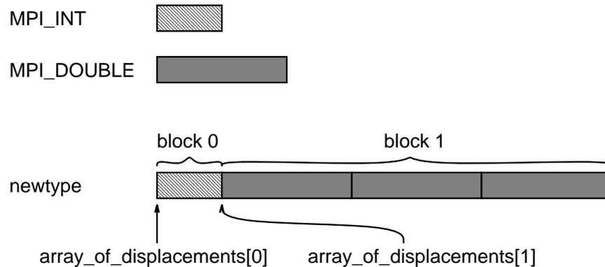
**Figure 28:** Illustration of a call to `MPI_TYPE_STRUCT` with `count = 2`, `array_of_blocklengths[0] = 1`, `array_of_types[0] = MPI_INT`, `array_of_blocklengths[1] = 3` and `array_of_types[1] = MPI_DOUBLE`
