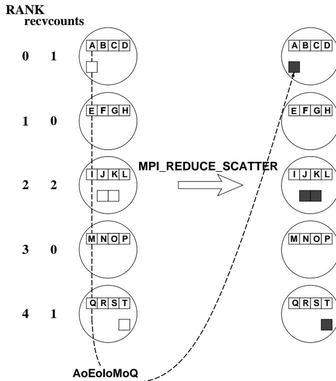
Figure 35: Global reduction in MPI with `MPI_REDUCE_SCATTER`. The symbols are as in Figure 33: The difference from `MPI_ALLREDUCE` is that processes elect to receive a certain-size segment of the result. The segments are always distributed in rank order.
