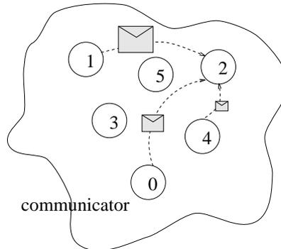
Figure 16: Processes can receive messages of different sizes.
