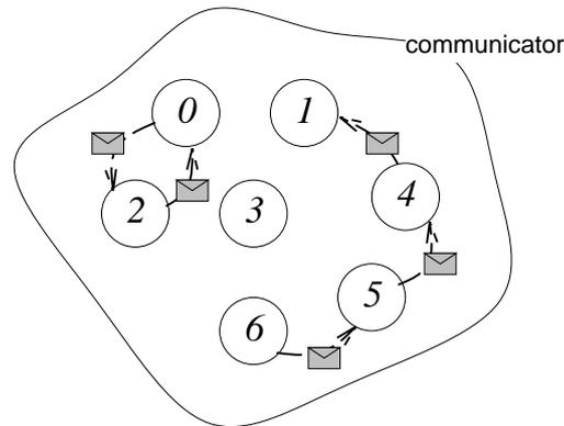
Figure 39: An example of two shifts. `MPI_SENDRECV` could be used for both
