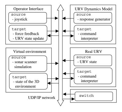
Fig.4. URV control and simulation system structure
