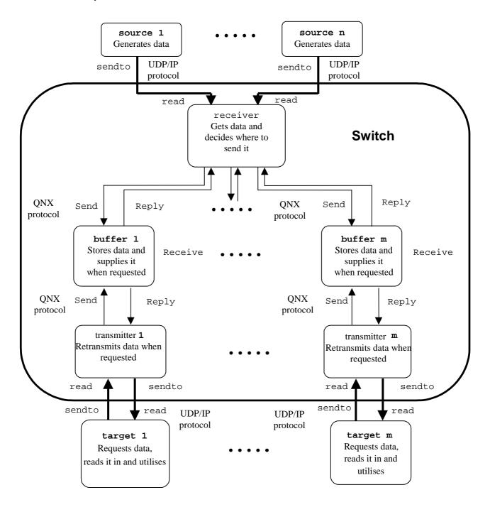
Fig.2 Internal Structure of the Communication Switch
