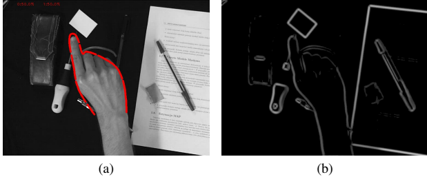
Fig. 8. Cluttered desktop environment used for evaluating tracker performance. (a) input grayscale image (b) edge image - the source of image observations
