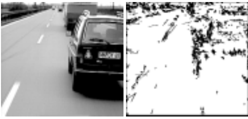
Figure 7.4 Real image (left) and the vector field for updated (v_x, v_y) motion.
