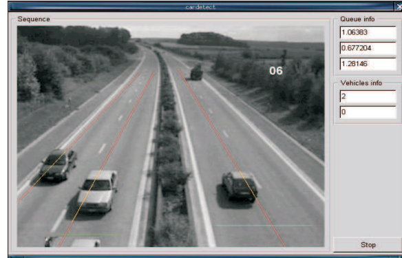
Figure 8. The queue lengths are detected and expressed numerically in terms of average car lengths, for each road lane under control.
