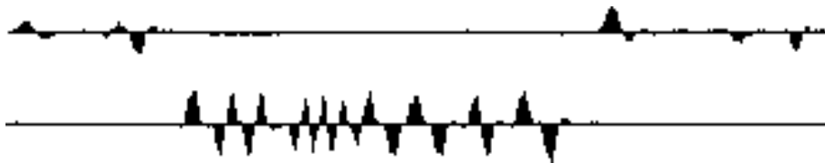
Figure 10. The idea of licence plate detection: the analysis of intensity distributions along image lines.
