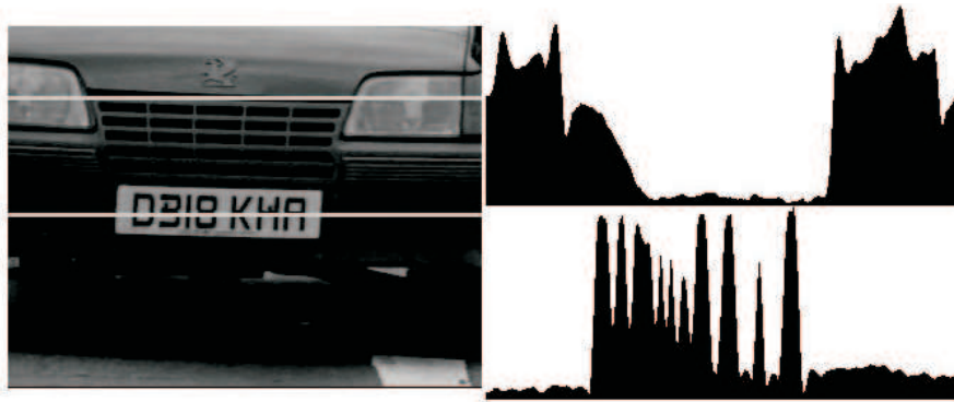
Figure 10. The idea of licence plate detection: the analysis of intensity distributions along image lines.
