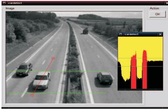
Figure 7. Example of queue length detection: the car detected in the lane on the left side causes two black and two light regions along the line of search.
