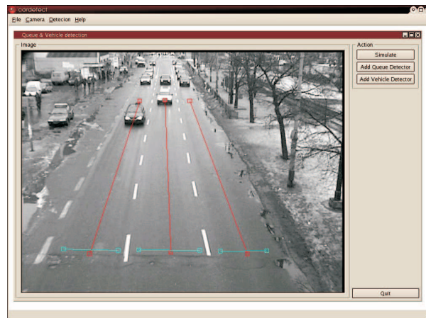
Figure 6. The horizontal lines represent two scan lines in the image, where the number of passing cars is counted. The vertical lines represent lanes, along which the queue lengths are detected.
